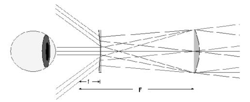
Figure 9.3: The ray diagram for Galileo's telescope.
