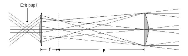
Figure 9.2: The ray diagram for Kepler's telescope.
