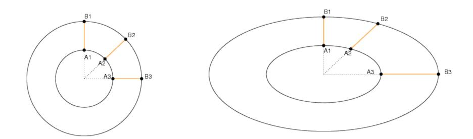
Elliptic streamlines have shear even in uniform rotation
