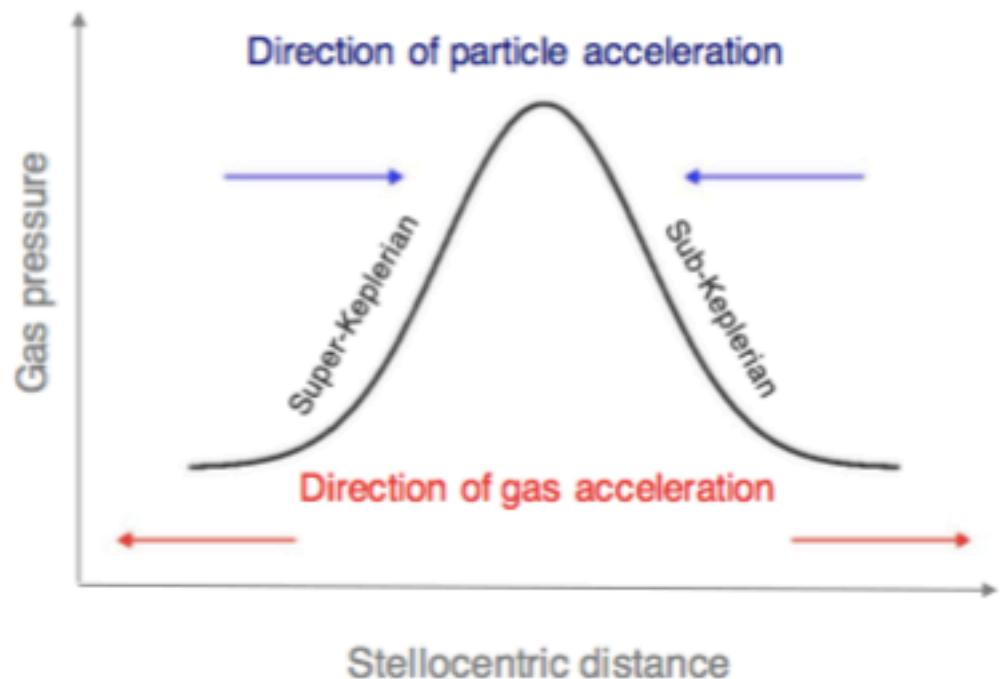
**Turbulence concentrates solids mechanically in pressure maxima**
