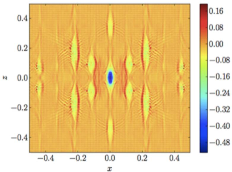
**Figure 1.** Vertical vorticity  $\omega_z$  in a  $x-z$  cut of our fiducial simulation with  $\text{Re}_6 = \text{Pe}_6 = 5 \times 10^5$  at  $t = 500$ . Similarly to [Marcus et al. 2013](#), we observe the formation and replication of anticyclonic vortices on a fixed lattice.
