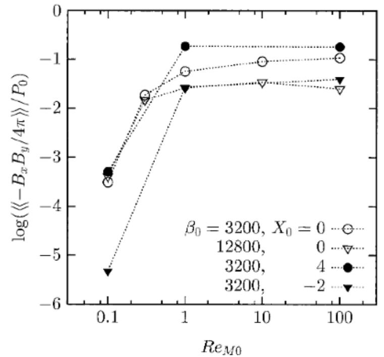
FIG. 9.—Saturation level of the Maxwell stress as a function of the magnetic Reynolds number  $Re_{M0}$ . Open circles and triangles denote the models without Hall term ( $X_0 = 0$ ) for  $\beta_0 = 3200$  and 12,800, respectively. The models including the Hall term are shown by filled circles ( $X_0 = 4$ ) and triangles ( $X_0 = -2$ ).
