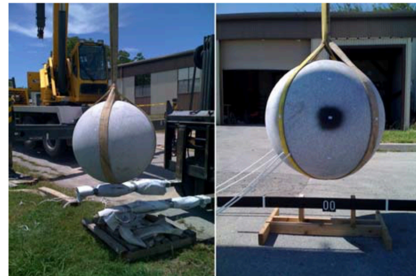
Figure 1. A 1-meter-diameter granite sphere suspended for the large-scale ‘pendulum’ experiments. Left: Placement of support strapping and lifting from forklift. Right: Sphere suspended in place for experiment with 1-meter scale bar and experiment run number marker shown.
