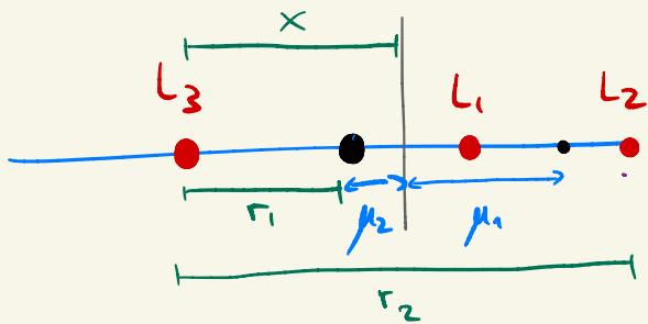
$$\mu_1 \left( -\frac{1}{r_1^2} + r_1 \right) \frac{(x + \mu_2)}{r_1} + \mu_2 \left( -\frac{1}{r_2^2} + r_2 \right) \frac{(x - \mu_1)}{r_2} = 0$$
