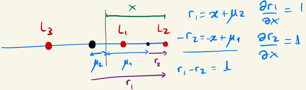
$$\mu_1 \left( -\frac{1}{r_1^2} + r_1 \right) \frac{(x + \mu_2)}{r_1} + \mu_2 \left( -\frac{1}{r_2^2} + r_2 \right) \frac{(x - \mu_1)}{r_2} = 0$$
