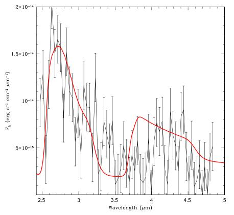
Figure 10. ISOPHT-S spectrum for AM Her. The red line is a cyclotron model with B = 12.8 MG. The cyclotron hump centered near 2.8  $\mu$  is due to the n = 3 harmonic, with n = 2 at 3.9  $\mu$ m.
