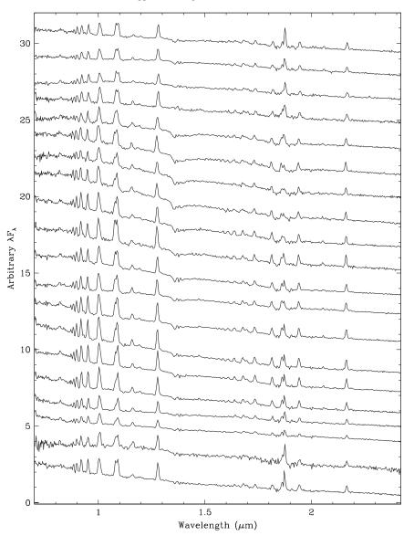
Figure 60. Near-IR spectra for V1432 Aql obtained with SpeX on the IRTF. These spectra have been phased using the ephemeris of Andronov et al. (2006), with the  $\phi = 0$  spectrum at the bottom, with the phase incremented by +0.05 vertically. The  $\phi = 0.05$  spectrum corresponds to the time of the eclipse, and we believe it was obtained closest to true phase zero.
