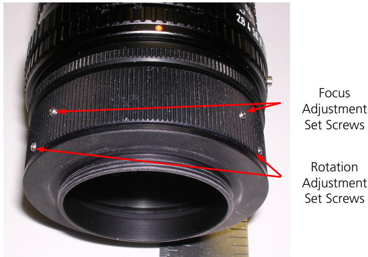
Figure 5. Location of lens adapter focus and rotation adjustment set screws.
