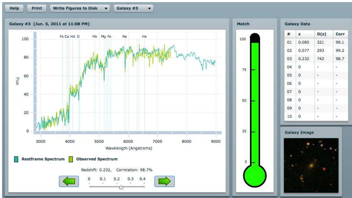
Figure 7.2: A screen capture of our galaxy spectrum analysis tool. Students determine galaxy redshifts by shifting the galaxy spectrum left and right in wavelength so as to match up absorption and emission features, as well as the general shape of the continuum, to a rest-frame spectrum of an equivalent galaxy. The correlation coefficient is reported numerically and also shown graphically on a symbolic thermometer – the better the match between the two spectra, the higher the level of the green “liquid” in the thermometer. The galaxy image in the lower right-hand corner has a constant angular size, so that galaxies that are further away from us appear smaller.
