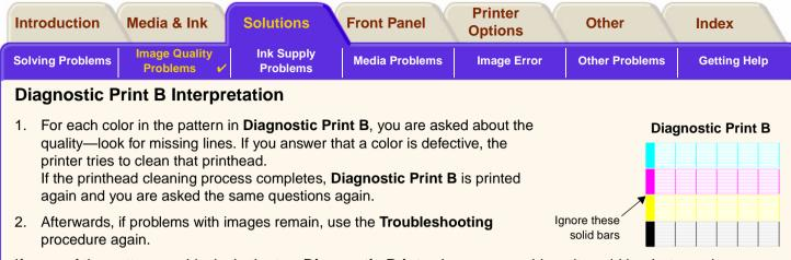
If none of the patterns or blocks in the two **Diagnostic Prints** shows any problem, it could be that your image quality problem is caused by a wrong setting in your software, or perhaps the job should have been printed with the **Print quality** set to **Best** instead of **Normal** or **Draft**.
