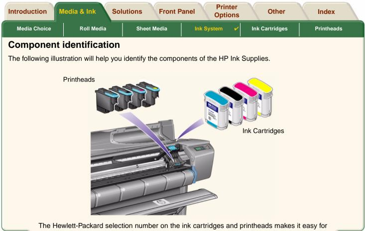
The Hewlett-Packard selection number on the ink cartridges and printheads makes it easy for you to find the correct HP Ink Supplies for your printer. Determine the color of the printhead or ink cartridge you need, then make sure you purchase or order the correct Hewlett-Packard printhead or ink cartridge. Each ink cartridge and printhead can be purchased separately from your usual Hewlett-Packard retailer. See <u>Ordering Accessories</u>.
