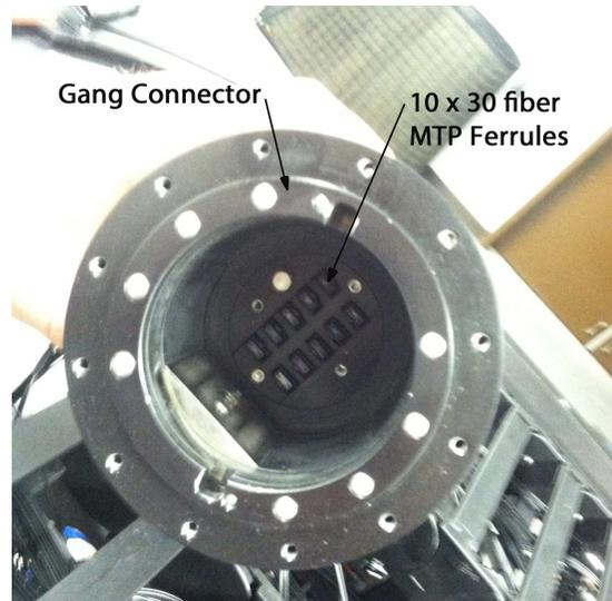
FIG. 10.— Receiving end of the APOGEE gang connector. A bayonet style connector slides into the bore and locks with a quarter turn. Ten 30 fiber MTP ferrules can be seen in an array inside the connector body.
