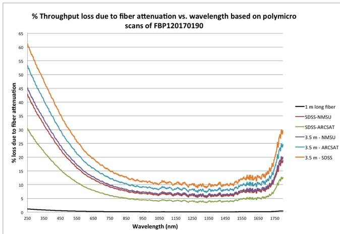
FIG. 12.— Expected percent throughput losses for fiber runs between the 4 telescopes at APO in the optical from  $\lambda = 250 - 1700$  nm. Values are based on an attenuation scan on fibers used for the BOSS spectrograph.
