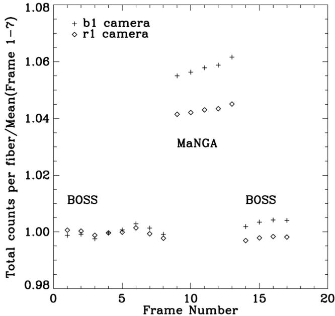
FIG. 9.— Comparison of the mean per fiber throughput between BOSS (W/O AR coating) single fibers and MaNGA (W/ AR-Coating) IFUs. As expected from the AR coating curve the MaNGA fibers perform about 4% better than the uncoated BOSS fibers. This shows a reduction in fresnel losses of about 1.5% for each air-glass interchange.
