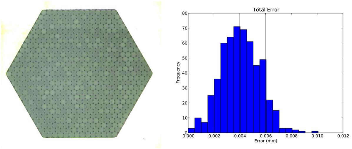
FIG. 15.— Left: 547 fiber IFU terminated into a tapered hexagonal stainless steel ferrule. Right: Distribution of fiber deviation from perfect placement within the IFU, vertical lines indicate the media error ( $4 \mu\text{m}$ ) and the 90% threshold error ( $6 \mu\text{m}$ )
