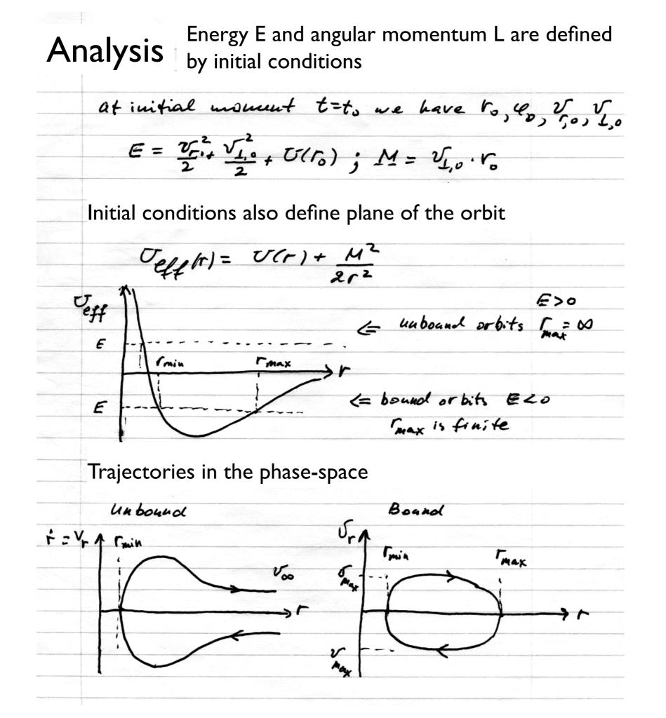
[max Gmin Trajectory always stays between Timin and Timax The radial period of the motion is agual to  $T_{p} = 2 \int \frac{d\sigma}{\sqrt{2(E - U_{eff}(r))}}$ During one period the apocenter drifts by angle  $\Delta \varphi = \chi \int \frac{\mu}{r^2} \frac{dr}{\sqrt{2(E-U_{eff})}}$ Trajectory is closed if sy= 25 m, where mange are integer numbers Orbits are alosed only in two cases: U(r) = A and U(r) = Ar2 If a trajectory is not close, it covers densily all the space between This and That
