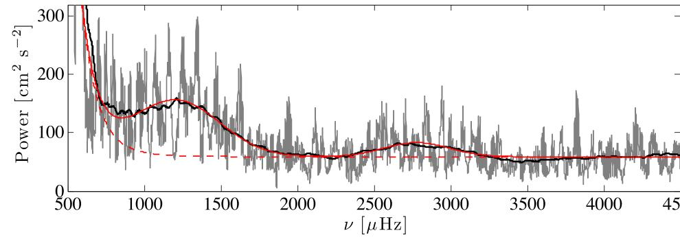
Above: evidence of the first detection of Jupiter's global modes from the SYMPA instrument, similar to the one to be built in this project. Excess oscillation power is detected between 800 and 3400  $\mu$ Hz, as well as a comb-like structure of regularly spaced peaks [from Gaulme et al. 2011].
